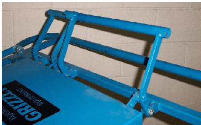
Fig. 8 Levers in brake on, clutch disengaged position
