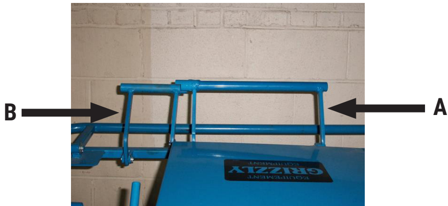
Fig. 3 : Power unit controls A- Clutch handle B- Brake handle
