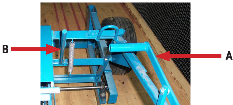
Fig. 4 A- Gravel dispensing lever B- Dump hopper released lever
