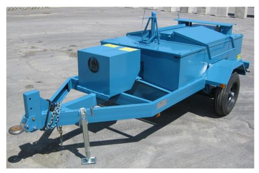
Industrial jack leg Stabilizer leg Silicon rubber sealed covers 1000° insulation
