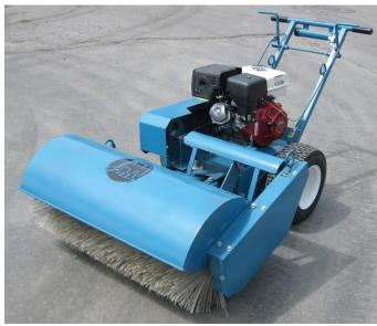
Independent and adjustable engagement of wheels and brush Differential with 1" axles
