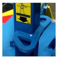
Travel restraint anchoring rings
