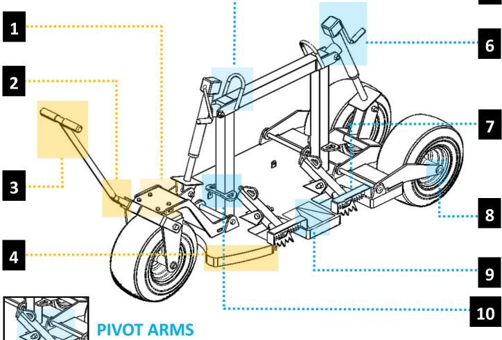
In fall arrest mode, the user must anchor his safety lanyard to one of the yellow pivot arms. The close proximity of the teeth and the roof deck will allow immediate engagement in case of a fall.
