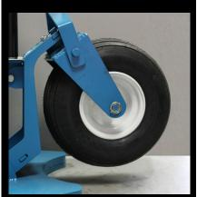
Secure the HERCULES Raising the wheels with the built-in jacks automatically immobilize the system.
