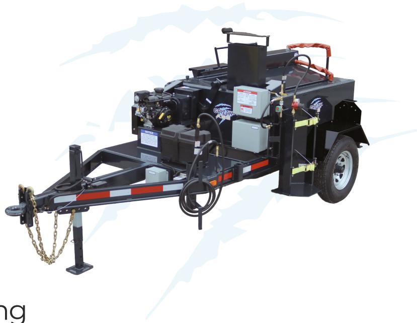
Fast, consistent melting with stable, oil-jacketed heat for reliable hot-pour performance.
