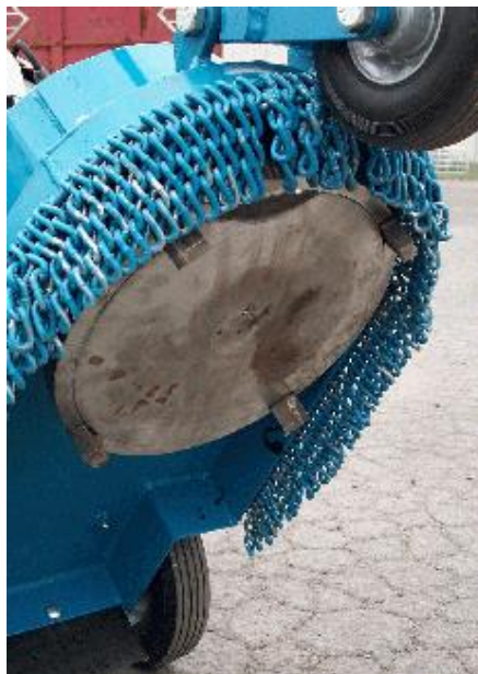
Fig. 7 Carbide blocks on disc planer
