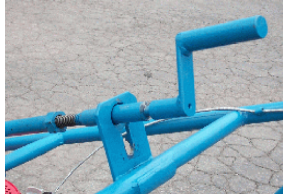
Fig. 5 Depth control in operation position
